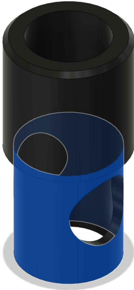
Insert both slider supports in the lower ball screw support (this can be done with the Z in place in the raised position - the below is for illustration purposes as alignment is important). The openings should be inline with the M6 Screw thread on the right side of the axis.
